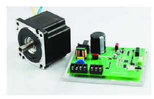
CASE 08 BLDC Motor Drive
